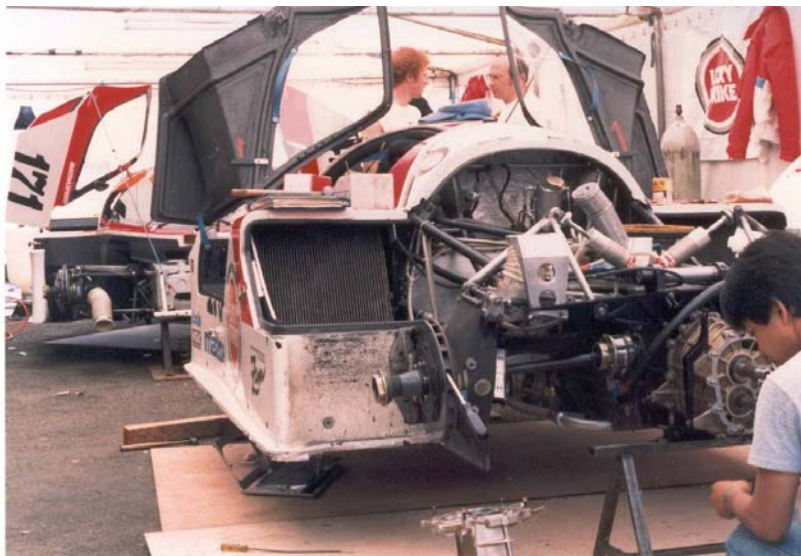
Le Mans 1986: Work on the Mazda 757 driven by Takashi Yorino, Yojiro Terada and Yoshimi Katayama. The car retired with a gearbox problem
